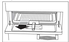
Remove the pan from the bottom of the broiler compartment.
